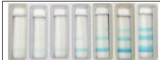
Figure 6. Demonstration of an enzyme-based ladder-bar assay for glucose detection (0, 1, 5, 25, 50, 100, and 200 \mu\text{M} ). The image is reprinted from Fung et al. 28 , Copyright (2009), with permission from Elsevier.
