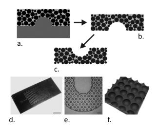
**Figure 1**. Fabrication of magnetite-PDMS structures. (a-c) The fabrication process. PDMS prepolymer is mixed with magnetite particles and cast over a suitable mold (a). After curing, the magnetite-PDMS is peeled off (b) and the surface PDMS etched back (c) to expose the embedded magnetite particles. (d and e) show an example of a microfluidic channel (50 μm deep) fabricated from magnetite-PDMS (1:1 particle:PDMS ratio). The mold used for casting this channel was fabricated as
