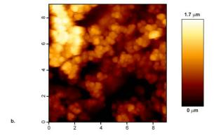
**Figure 2.** SEM and AFM characterization of magnetite-PDMS substrates. (a) SEM images taken at x400 and x10,000 magnification of three substrates with different magnetite:PDMS ratios. (b) A typical AFM image of 1:1 magnetite-PDMS substrate.
