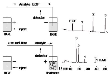
A simple approach to zero net-flow in electrophoresis using acrylamide based hydrogel at one end of the capillary is described.
