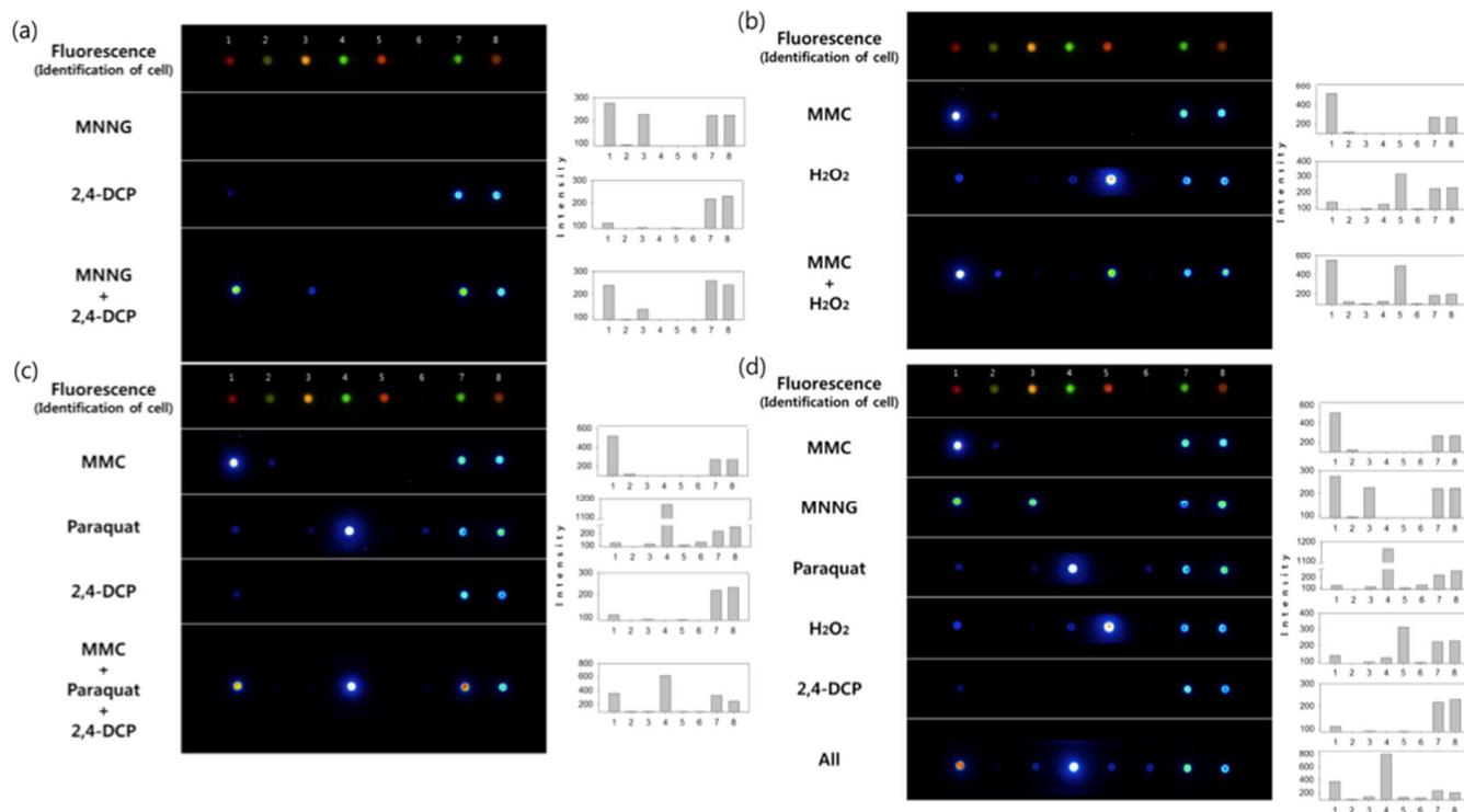
**Figure 2.** Bioluminescent data of Multiple-dose test using mixed chemical. (a) MMC 2 ppm and Paraquat 25 ppm (b) MNNG 2 ppm and 2,4-DCP 30 ppm (c) MMC 2 ppm, Paraquat 25 ppm and 2,4-DCP 30 ppm (d) All chemical (MMC 2 ppm, MNNG 2 ppm, Paraquat 25 ppm, H<sub>2</sub>O<sub>2</sub> 17 ppm and 2,4-DCP 30 ppm).
