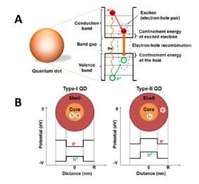
**Figure 3. Electrical properties of quantum dots.** (A) Illustration of electron-hole recombination and corresponding energy levels. (B) Energy level diagram of type-I and type-II QDs.
