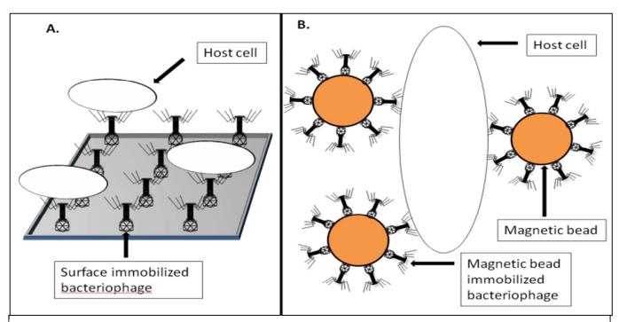
**Figure 3. Bacteriophage biosorbents.** (A) Surface immobilized bacteriophage biosorbent for specific host capture. (B) Magnetic bead immobilized bacteriophage biosorbent for specific host capture.
