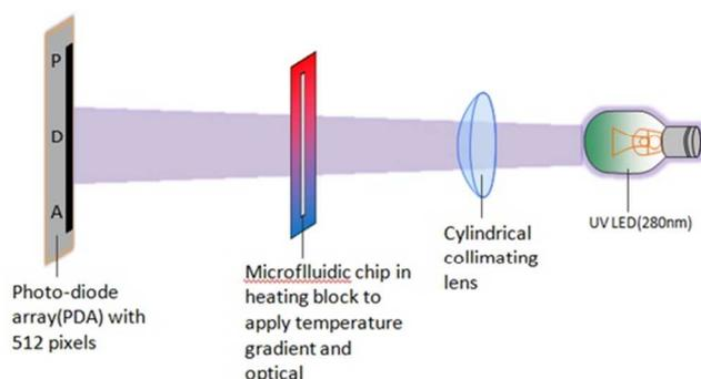
**Fig.2** Schematic of optical setup.
