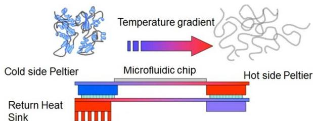
**Fig.1** Schematic of thermal setup.
