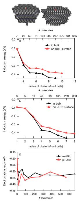
**Figure 4**: A: Space-filling model of  $\alpha$  (left) and  $\beta$  (right) phthalocyanine clusters. B: Induction interaction of a positive charge in  $\alpha$ -phthalocyanine in the bulk and on the surface. C: Induction interaction of a positive
