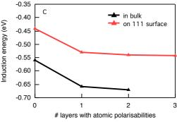
Figure 2: A: Schematic representation of a hemispherical  $C_{60}$  cluster with a central negatively charged molecule (in red); B: Induction energy as a function of cluster size for the  $C_{60}$  surface and bulk in the atomic and molecular polarisability description; C: Effect of combining the atomic and molecular polarisability descriptions.
