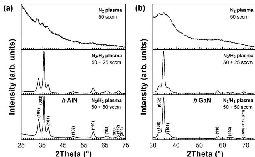
**Fig. 10** GIXRD patterns of (a) AlN, and (b) GaN thin films deposited on Si (100) substrates using N<sub>2</sub>/H<sub>2</sub> (50 + 50 sccm), N<sub>2</sub>/H<sub>2</sub> (50 + 25 sccm), and N<sub>2</sub> (50 sccm) plasma.
