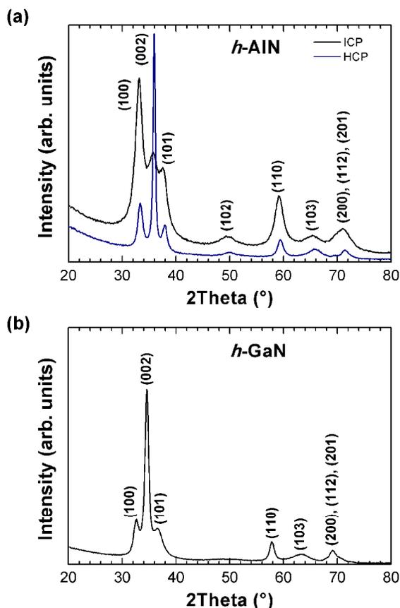
**Fig. 2** GIXRD patterns of (a) AlN, and (b) GaN thin films deposited on Si(100) substrates using  $\text{NH}_3$  plasma. GIXRD pattern of the AlN thin film deposited using quartz-based ICP source<sup>21</sup> is also shown in (a) for comparison.
