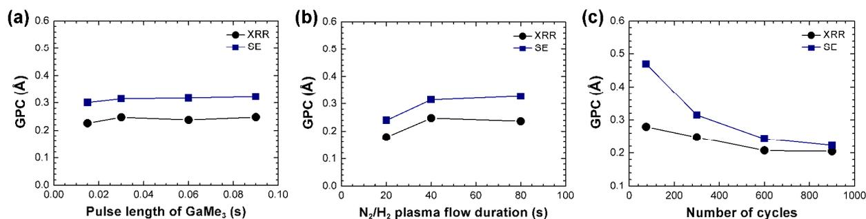
**Fig. 5** (a) GaMe<sub>3</sub>, and (b) N<sub>2</sub>/H<sub>2</sub> saturation curves at 200 °C. For the GaMe<sub>3</sub> saturation curve, N<sub>2</sub>/H<sub>2</sub> flow rate and flow duration were kept constant at 50 + 50 sccm and 40 s, respectively. GaMe<sub>3</sub> pulse length was 0.03 s for the N<sub>2</sub>/H<sub>2</sub> saturation curve. (c) GPC plotted as a function of number of deposition cycles. Data suggests substrate-enhanced growth of GaN thin films.
