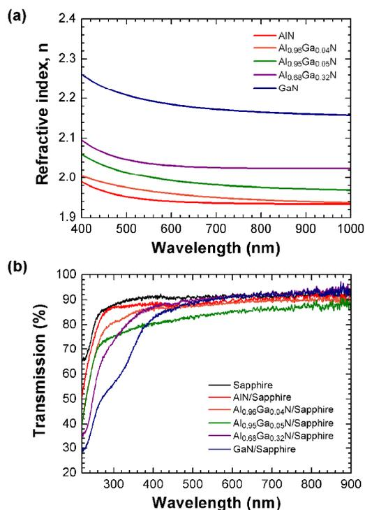
**Fig. 13** (a) Spectral refractive indices, and (b) optical transmission spectra of AlN, GaN, and Al<sub>x</sub>Ga<sub>1-x</sub>N thin films deposited on Si (100) and double side polished  $c$ -plane sapphire substrates, respectively.
