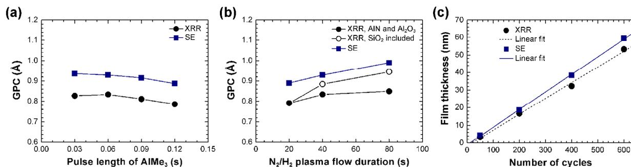
**Fig. 4** (a) AlMe<sub>3</sub>, and (b) N<sub>2</sub>/H<sub>2</sub> saturation curves at 200 °C. For the AlMe<sub>3</sub> saturation curve, N<sub>2</sub>/H<sub>2</sub> flow rate and flow duration were kept constant at 50 + 50 sccm and 40 s, respectively. AlMe<sub>3</sub> pulse length was 0.06 s for the N<sub>2</sub>/H<sub>2</sub> saturation curve. (c) AlN film thickness plotted as a function of number of deposition cycles.
