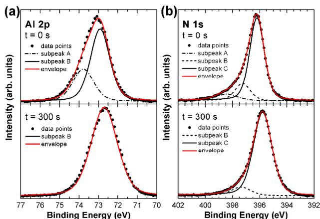
Fig. 6 (a) Al 2p, and (b) N 1s HR-XPS scans of 59.2-nm-thick AlN thin film deposited on Si (100) substrate using optimized HCPA-ALD parameters.
