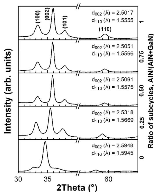
**Fig. 11** GIXRD patterns of AlN, GaN, and Al<sub>x</sub>Ga<sub>1-x</sub>N thin films deposited on Si (100) substrates.
