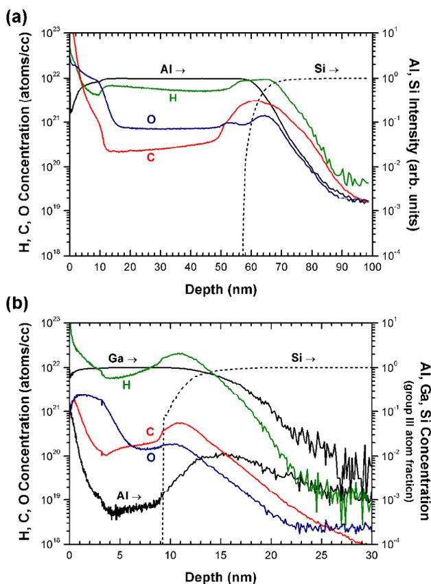
**Fig. 1** Impurity concentrations determined by SIMS depth profiling for (a) AlN, and (b) GaN thin films deposited using  $\text{NH}_3$  plasma. Silicon is not quantified in the layers, only plotted as the substrate layer marker.
