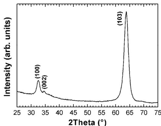
Fig. 8 GIXRD pattern of 20.1-nm-thick GaN thin film deposited on *c*-plane sapphire substrate using optimized HCPA-ALD parameters.
