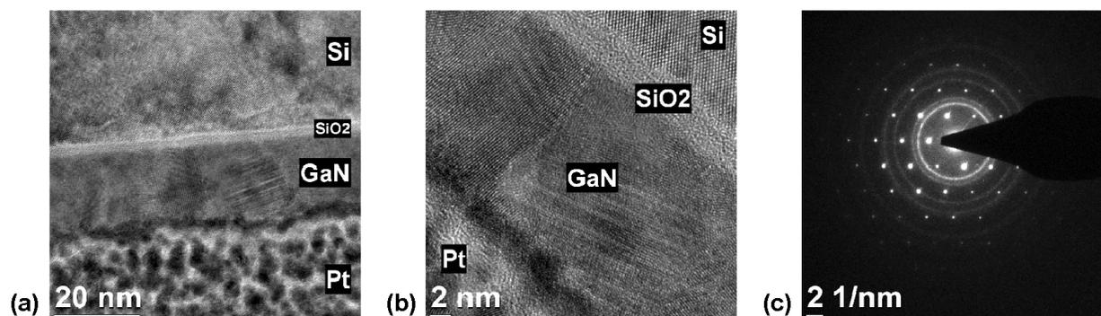
**Fig. 3** Cross-sectional (a) TEM, and (b) HR-TEM images of 21-nm-thick GaN thin film deposited on Si (100) substrate using NH<sub>3</sub> plasma. FIB-induced SiO<sub>2</sub> damage layer formed at the GaN/Si interface during TEM sample preparation. (c) SAED pattern of the same sample.
