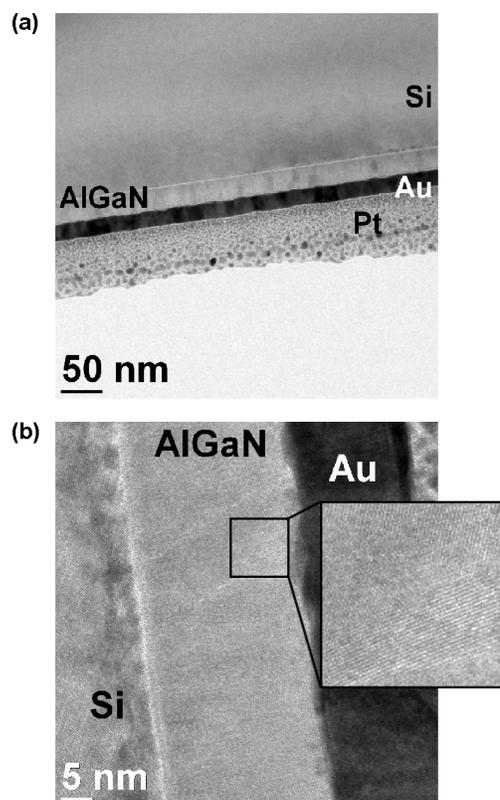
**Fig. 12** Cross-sectional (a) bright-field STEM, and (b) HR-TEM images of 25.4-nm-thick Al<sub>0.68</sub>Ga<sub>0.32</sub>N thin film deposited on Si (111) substrate using N<sub>2</sub>/H<sub>2</sub> plasma.
