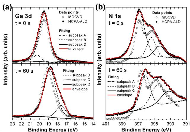
Fig. 7 (a) Ga 3d, and (b) N 1s HR-XPS scans of 20.1-nm-thick GaN thin film deposited on Si (100) substrate using optimized HCPA-ALD parameters.
