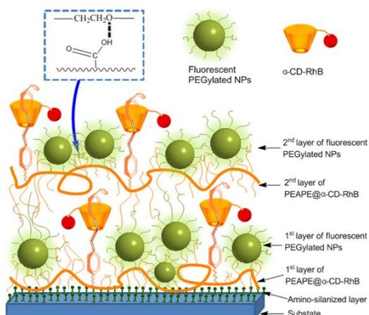
Scheme 1 Schematic expression of PEGylated NPs-azobenzenes LbL self-assembly at quartz wafer surfaces. The inset illustrates the H-bonding between the carboxylic groups of PEAPE and other groups of MePEG.
