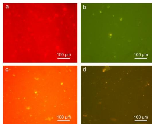
Fig. 2 Fluorescent microphotographs of PEAPE@ $\alpha$ -CD-RhB/unlabeled NPs (a), PEAPE/labelled NPs (b) multilayers, multicolor fluorescence film before (c) and after (d) UV irradiation. The size bar is 100  $\mu\text{m}$ .
