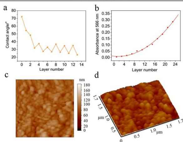
Fig. 1 Multilayer growth characterization. Water contact angles as a function of layer number (a) and absorbance at 566 nm vs. the layer number (b). AFM (c and d) images of 6-bilayer film deposited on a quartz wafer. Scan in  $1.7 \mu\text{m} \times 1.7 \mu\text{m} \times 180 \text{nm}$ .
