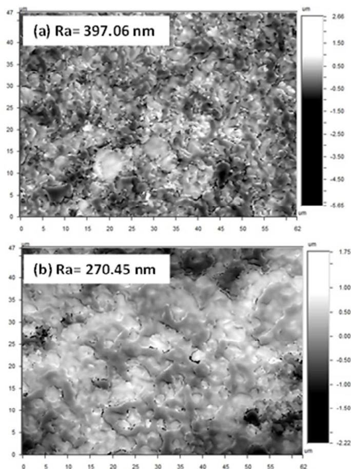
**Fig. 3** Profilometry images and average roughness of (a) Bare SPCE; (b) single layer PPy film on SPCE.
