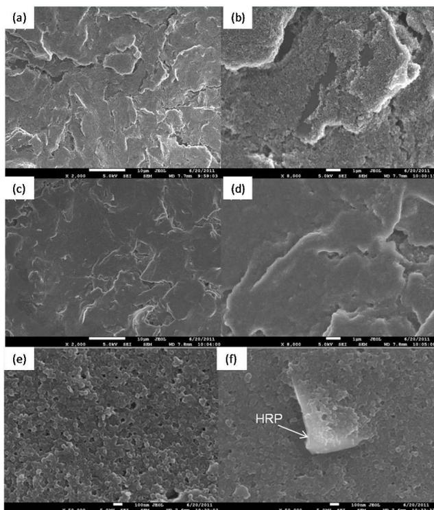
**Fig. 2** (a) SEM image of bare SPCE, scale bar: 10  $\mu\text{m}$ ; (b) SEM image of bare SPCE, scale bar 1  $\mu\text{m}$ ; (c) SEM image of one layer of PPy film on SPCE, scale bar, 10  $\mu\text{m}$ ; (d) SEM image of one layer of PPy film on SPCE, scale bar, 1  $\mu\text{m}$ ; (e) PPy nanoparticles that constituted 1 layer PPy/HRP film, scale bar: 100 nm; (f) Detail of PPy particles encapsulating HRP enzyme crystal, scale bar 100 nm.
