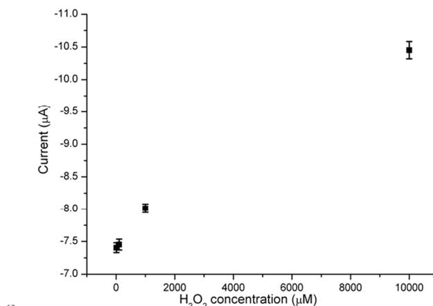
Fig. 5 The reproducibility calibration curve of five single layer inkjet printed PPy/HRP biosensors. Error bars represent RSD of single measurement of five sensors.
