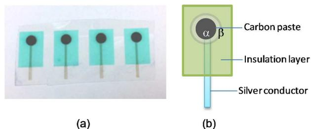
**Fig. 1** (a) Strip of four bare SPCEs on Polyethylene terephthalate (PET); (b) Schematic of the inkjet printed PPy/enzyme biosensor based on an SPCE. (α) inner black circle: PPy/enzyme film on carbon paste (diameter: 5.5 mm); (β) outer white circle covering inner black circle: EC membrane covering PPy/enzyme electrode (diameter: 7 mm).
