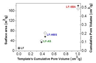
Fig. 6 Correlation between the specific surface area (large empty 20 rhombs) and the cumulative pore volume (small full rhombs) of LaFeO<sub>3</sub>based nanopowders with the cumulative pore volume of the original silica template.
