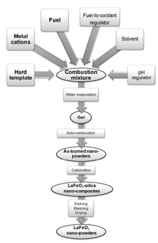
Scheme 1 Step-by-step description of the experimental procedure used in the SHT approach.
