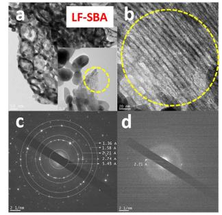
Fig. 10 (a) TEM images of LF-SBA powder, where the inset evidences the presence of a poorly crystalline region (yellow circle); (b) <sup>45</sup> TEM image of the poorly crystalline region; (c) diffraction patterns of the crystalline region and (d) diffraction patterns of the poorly crystalline region.
