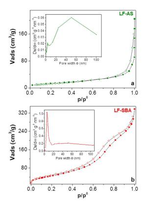
Fig. 5 Sorption isotherms and pore size distribution of LF-AS (a) and LF-SBA (b).
