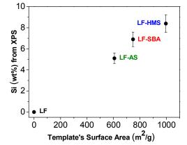
65 Fig. 8 Surface Si wt% calculated from XPS analysis as a function of the silica templates' specific surface area. Error bars are also reported in the graphic.
