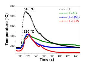
Fig. 1 Temperature/time profiles recorded during the combustion process of LaFeO<sub>3</sub>-based nanopowders prepared with (full lines with squares/AS, triangles/HMS or circles/SBA) and without (dotted line with stars) silica templates.
