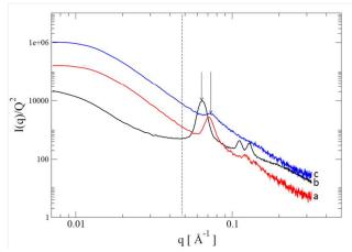
Fig. 12 The continuous black (a), red (b) and blue (c) lines are the SBA-15, the LF-SBA<sub>BE</sub> (before etching) and the LF-SBA final powder, respectively. The arrows indicate the shift toward higher q values of the LF-SBA with respect to the original SBA-15 hard template.
