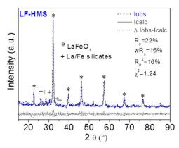
25 Fig. 4 Graphical Rietveld fit of LF-HMS after thermal treatment at 800°C/48h. Reliability factors are also reported in the figure.
