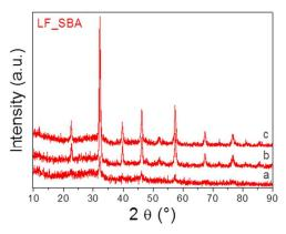
Fig. 2 XRD patterns of LF-SBA samples a) as-burned, (b) after calcinations at 700C for 5h before etching and (c) after etching with NaOH.
