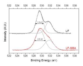
Fig. 9 Comparison between the O 1s XPS spectra of LF and LF-SBA nanopowders.
