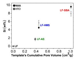
Fig. 7 Bulk Si wt% measured by neutron absorption analysis (large full circles) and determined from X-ray diffraction (small empty circles),
