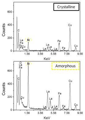
Fig. 11 Elemental analysis (EDX spectra) of crystalline and amorphous components of LaFeO<sub>3</sub>-based nanopowders prepared using 50 the SBA-15 silica template
