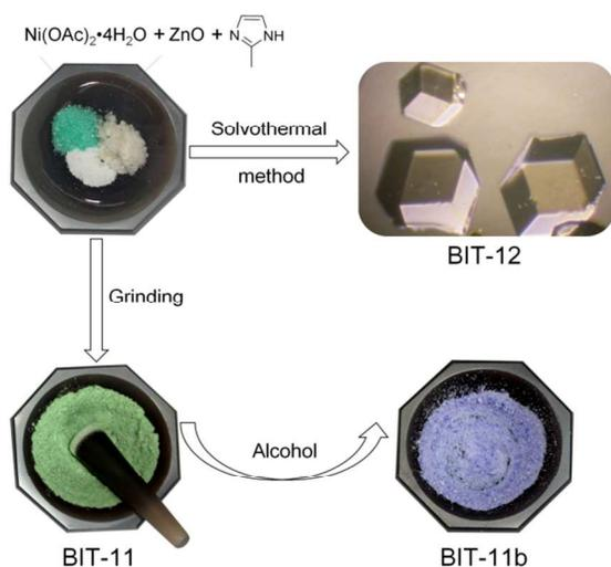
**Fig. 1** Schematic representation of the mechanochemical synthesis of BIT-11 and -11b, as well as the microscopic photo of BIT-12 single crystals synthesized solvothermally.
