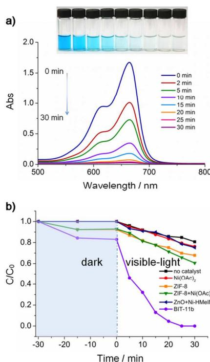
**Fig. 5** (a) UV-vis absorption spectra of MB solution degradation by BIT-11b under visible-light irradiation for different time intervals. The insert photograph highlights the experiment result of photodegradation, from left to right: MB solution, 0 min, 2 min, 5 min, 10 min, 15 min, 20 min, 25 min, 30 min. (b) Comparison of photocatalytic performance of MB degradation on samples under visible-light irradiation. ( $C_0=10 \text{ mg/L}$ ,  $100 \text{ mL}$ ; the weight of catalyst = 20 mg).
