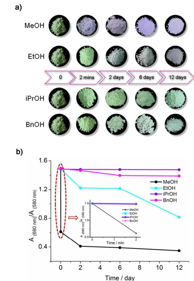
**Fig. 4** (a) The pictures of the apparent color changes for BIT-11 soaked in different alcohols at certain time intervals. (b) Absorption data of  $A_{680}/A_{580}$  for BIT-11 upon soaking in variable alcohols over the time.
