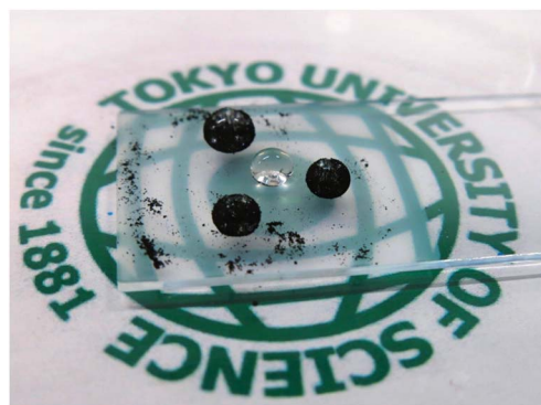
Fig. 7 The self-cleaning behavior of the superhydrophobic coatings prepared from 2 vol% of PMMA in silica at a deposition time of 30 min.
