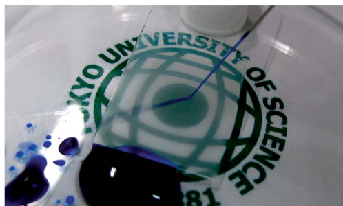
Fig. 8 Water jet impact study on the superhydrophobic coatings prepared from 2 vol% of PMMA in silica at a deposition time of 30 min.
