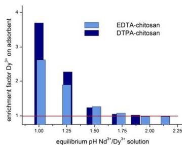
Dysprosium is enriched in comparison with neodymium at low pH values on EDTA- and DTPA-functionalized chitosan. The observed differences in selectivity are used to separate mixtures of rare earths by column chromatography.
