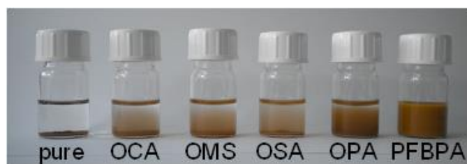
Figure 4. Photographs of dispersions in DMF of pure and various modified CCTO particles.
