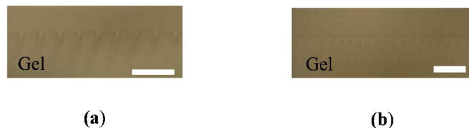
Figure S4: Optical micrographs (scale bar 100 \mu\text{m} ) of gel ( E \sim 23 kPa) filled PDMS master prior to molding for periodic ridge geometry (a) h \sim 13 \mu\text{m} , \lambda \sim 35 \mu\text{m} and (a) h \sim 2.7 \mu\text{m} , \lambda \sim 25 \mu\text{m}
