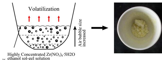
**Fig. 1** Schematic representation of the reaction process and the photo of synthesized porous ZrO<sub>2</sub> sample. (a) A illustration of the pore-forming mechanism. The precursor has been concentrated to a very high level, creating a liquid of poor flowability. Air bubbles (with a small size) in this circumstance will be frozen and aggregated where they were created. (b) A photo of amorphous ZrO<sub>2</sub> gels formed at 90 °C.
