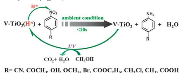
**Fig. 12** Schematic diagram for selective hydrogenation of nitroarenes to aminoarenes by  $\text{V-TiO}_2(\text{H}^*)$  and the regeneration process of  $\text{V-TiO}_2(\text{H}^*)$ . The active hydrogen ( $\text{H}^*$ ) in our material is not molecular hydrogen but a proton with an electron in its vicinity.<sup>42</sup> Reproduced by permission of The Royal Society of Chemistry.
