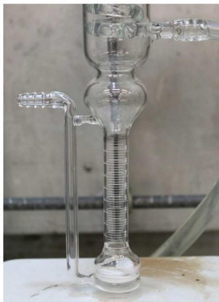
**Figure 15.** Carbon dioxide additional cell used to convert two phases of amine and water to a single phase polar SPS, **1'** through **16'**.
