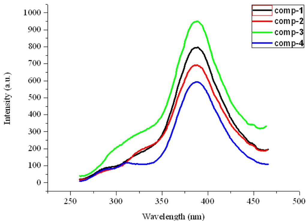
**Figure 7** Solid-state emission spectra for complexes **1–4**.
