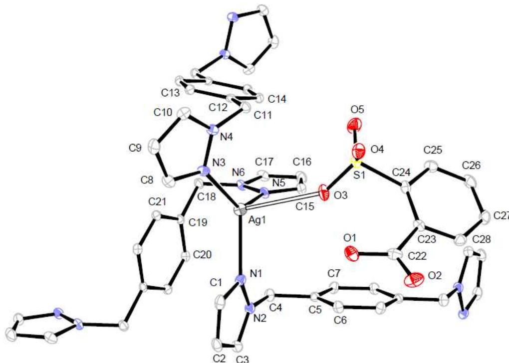
**Figure 2** ORTEP view of the asymmetric unit of complex **2** with the numbering scheme. The thermal ellipsoids are drawn at 30% probability. The weak bond is represented as open line. The H atoms are omitted for clarity.
