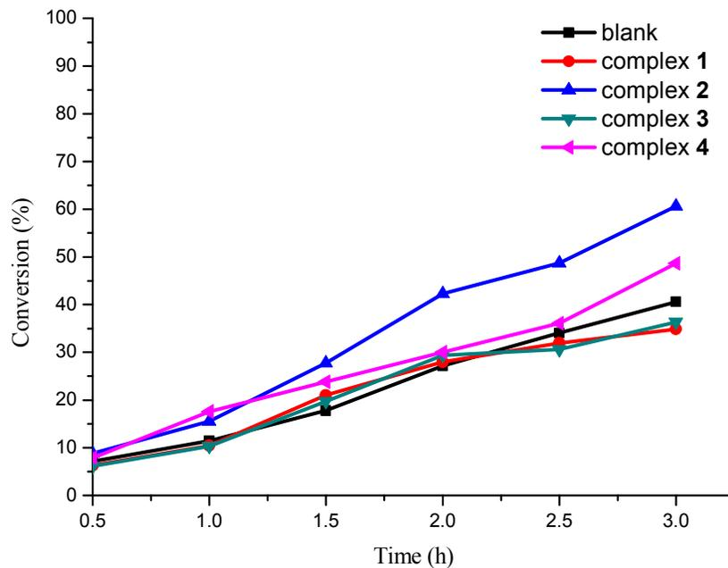
**Figure 8** The conversion of MPS vs reaction time plot for the oxidation of MPS by complexes 1-4. Blank experimental conditions: 0.5 mmol of MPS and 1.5 mmol of  $\text{H}_2\text{O}_2$  were mixed in 5 mL of ethanol at  $50^\circ\text{C}$ . The representative GC chromatograms are presented in Supporting Information (Figures S15-21).
