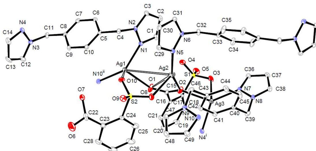
**Figure 1** ORTEP view of the asymmetric unit of complex **1** with numbering scheme and the probability is drawn at 30%. The H atoms and lattice water molecule are omitted for clarity. Symmetry codes, i:  $-1+x, 1+y, z$ ; ii:  $1+x, y, z$ .
