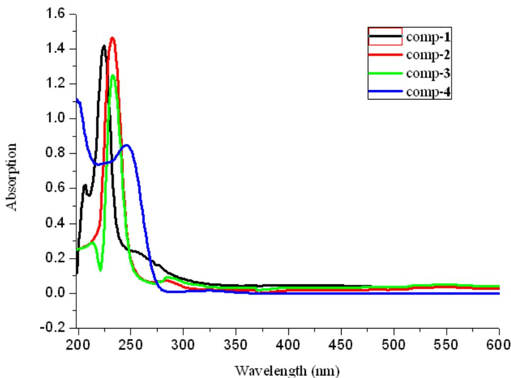
**Figure 6** UV-vis spectra of complexes **1–4** in methanol.
