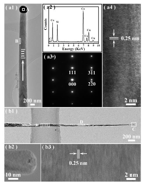
Fig. 2 (a1) A typical TEM image of the wire tip of S15 under a low magnification. (a2) A representative EDS spectrum recorded from the catalytic particle. (a3-a4) The corresponding SAED pattern and HRTEM image of the wire body of S15. (b1-b2) Typical TEM images of the wire tip of S20 under different magnifications. (b3) The corresponding HRTEM image of the wire body of S20.
