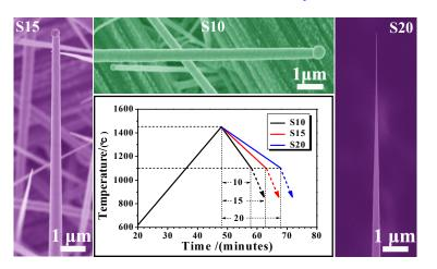
We report the controlled growth of 3*C*-SiC flexible field emitters with clear and sharp tips based on the VLS mechanism.
