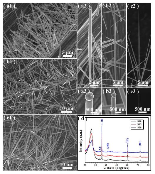
**Fig. 1** Typical SEM images of as-grown quasialigned SiC nanoarrays of S10 (a1, a2, a3), S15 (b1, b2, b3) and S20 (c1, c2, c3) under different magnifications. (d) Typical XRD pattern of the as-synthesized products of S10, S15 and S20.
