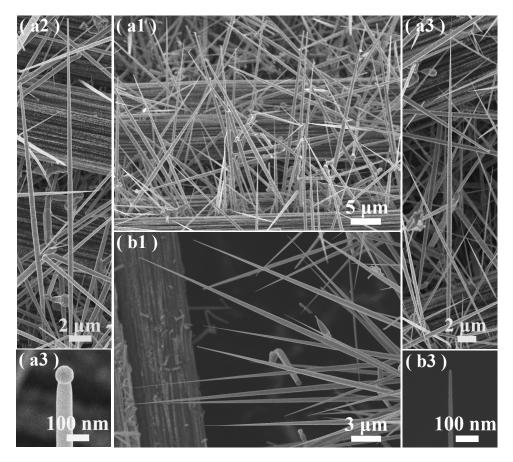
**Fig. 4** Typical SEM images of as-synthesized quasialigned SiC nanoarrays of S18 (a1, a2, a3) and S25 (b1, b2, b3) under different magnifications.
