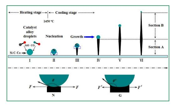
Fig. 3 Schematic illustration for the growth of SiC nanowires with tailored sharp tips based on the VLS mechanism.
