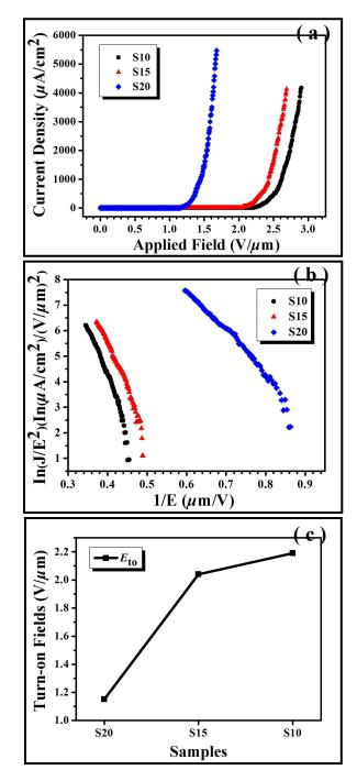
**Fig. 5** FE properties of the resultant Samples of S10, S15 and S20. (a) *J*-*E* plots of obtained three samples; (b) Corresponding F-N plots of three samples; (c) The variation of  $E_{to}$  of three samples.
