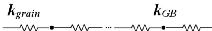
Fig. 1A- Line conductors in series with equal length connected with point conductors.
