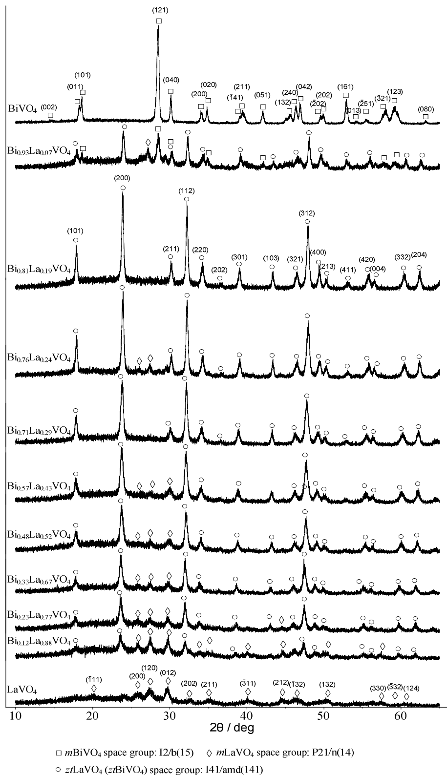
Fig. 1. XRD diffractograms for the \text{Bi}_x\text{La}_{1-x}\text{VO}_4 samples.
