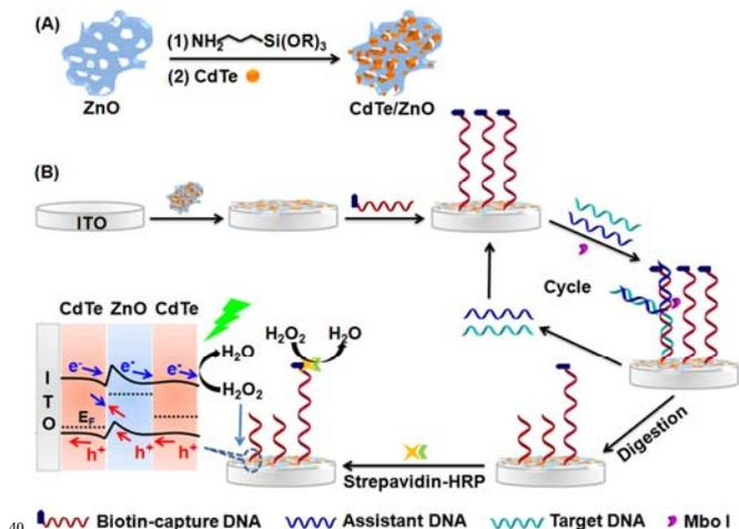
**Scheme 1** Schematic representation of (A) the synthesis of CdTe/ZnO nanohybrids, and (B) the construction and photoelectrochemical strategy of DNA biosensor.
