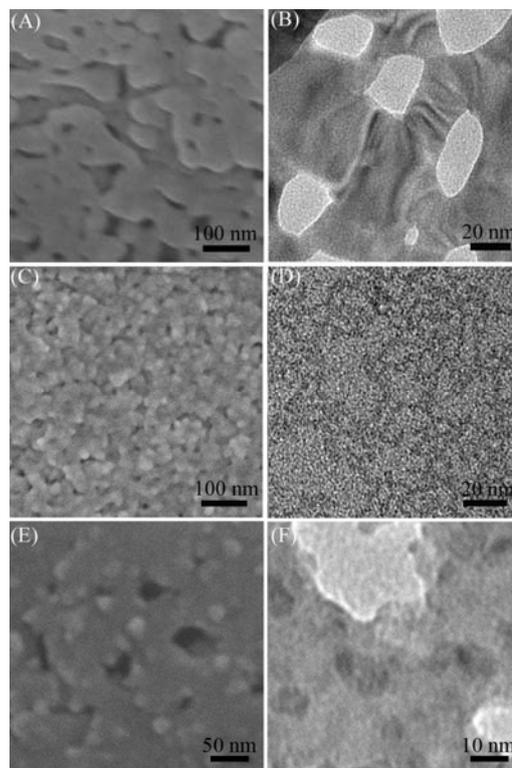
80 **Fig. 1** High resolution SEM and TEM images of (A) and (B) porous ZnO nanosheets, (C) and (D) CdTe QDs, and (E) and (F) CdTe/ZnO nanohybrids.
