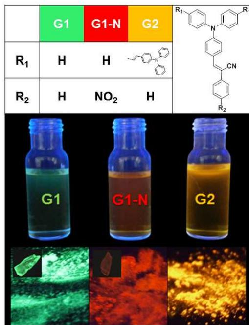
New triphenylamine substituted cyanostyrene luminogens (G1, G1-N and G2) with aggregation-induced emission (AIE) were synthesized.
