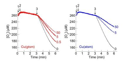
2 Figure 4. Inhibition electron transfer succinate of via dehydrogenase. Succinate-dependent consumption of O2 by cell-free membrane vesicles after pre-3 4 incubation with 0-50 µM each of Cu(gtsm) (red traces) or Cu(atsm) (blue traces). Addition 5 of membrane vesicles (1), DMSO or Cu compounds (2), and succinate (3) are indicated by 6 downward arrows. Representative results of at least three independent replicates are 7 shown.
