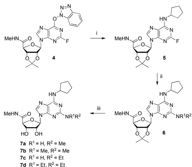
**Scheme 2.** Reagents and conditions: (i) CyclopentylNH<sub>2</sub>, *t*-BuOH, DIPEA, 80 °C; (ii) R<sub>2</sub>NH or RNH<sub>2</sub>, *t*-BuOH, 150 °C (iii) MeCN/1M HCl (4:1), 60 °C, 48–72%.
