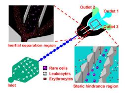
We present a multistage microfluidic device for continuous label-free separation of rare cells using a combination of inertial microfluidics and steric hindrance.
