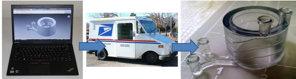
We explore the three-dimensional capabilities, resolution, and optical clarity of microfluidic devices fabricated by stereolithography using a mail-order service, and we compare the cost and prototyping speed of soft lithography with those of stereolithography.
