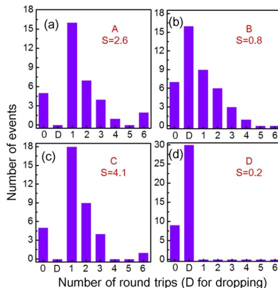
**Fig. 6** (a)-(d) Summary of  $2.2\mu\text{m}$  particle transport processes on A - D at on-resonance wavelengths. All particles are routed from the input-waveguide. The "0" bin: particle escaping without completing one round trip. The "D" bin: particle dropping.
