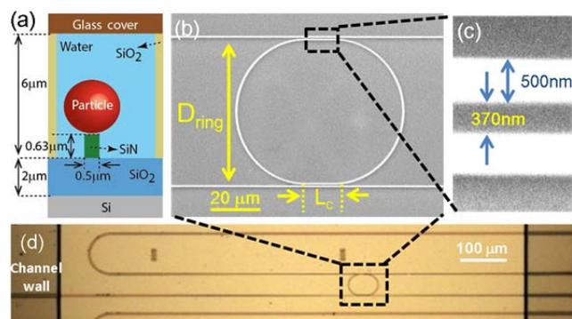
**Fig. 2** (a) Schematic cross-sectional view of the optofluidic chip with a trapped microparticle. (b) Top-view SEM image of the fabricated microring-resonator-based add-drop device.  $D_{\text{ring}}$ : arc diameter,  $L_c$ : interaction length. (c) Zoom-in-view SEM image of the coupling gap. (d) Top-view optical micrograph of the fabricated optofluidic chip with air-cladding.
