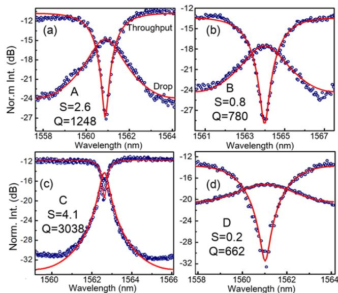
**Fig. 3** (a)-(d) Measured and fitted throughput- and drop-transmission spectra of (a) A, (b) B, (c) C and (d) D. Blue circles: data. Red lines: fitting according to transfer-matrix modelling.
