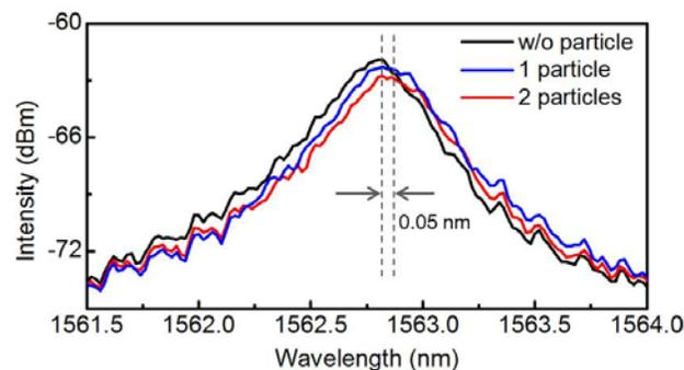
**Fig. 5** Measured drop-port transmission spectra of C upon zero, one and two trapped  $2.2\mu\text{m}$  particles.
