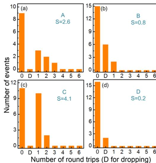
**Fig. 7** (a)-(d) Summary of  $0.84\mu\text{m}$  particle transport processes on A - D at on-resonance wavelengths. All particles are routed from the input-waveguide. The "0" bin: particle escaping without completing one round trip. The "D" bin: particle dropping.
