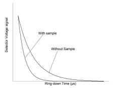
**Figure 1:** Ring-down trace showing exponential decay of the optical signal with and without analyte gas.
