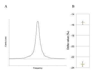
Figure 2: Panel A: Loss spectrum from WS-CRDS. The curve represents the cavity loss over a spectral line for a single analyte, for example <sup>13</sup>CO<sub>2</sub>. Panel B: Box plot of the analyzer delta value precision for two reference samples.
