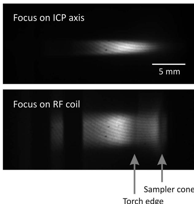
Fig. 1 Sodium atomic emission captured with the system focused onto the central channel of the plasma (top image) and onto the RF coil (bottom image). The bottom image was used for size calibration taking into account the width of the RF coil (3 mm), which is well visible on the left. On the bottom image, the edge of the quartz torch can be seen at about two third of the image from the left as well as the sampler cone at the end of the bright area.
