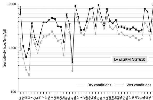
Fig. 7 Abundance-corrected sensitivities of elements measured by LA-ICP-QMS of SRM NIST 610 using wet and dry plasma conditions. The sensitivity pattern for the rare earth elements is unusual but is, most likely, due to an incomplete vaporization of micrometer sized particles which are known to be formed during LA at a wavelength of 266 nm, as performed here.
