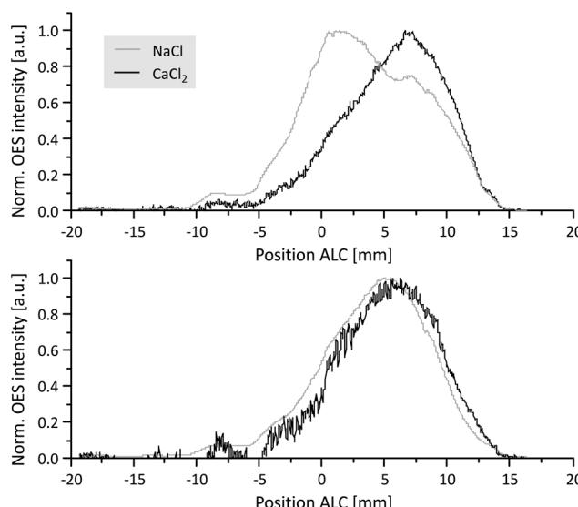
Fig. 4 Central axial emission profiles acquired for LA of sodium chloride and calcium chloride under dry plasma conditions (top panel) and during the addition of water using a concentric nebulizer (bottom panel). The profiles were integrated over a width of 4 mm and normalized with respect to maximum intensity values for better comparison. Positions are given as millimeter above load coil (ALC).
