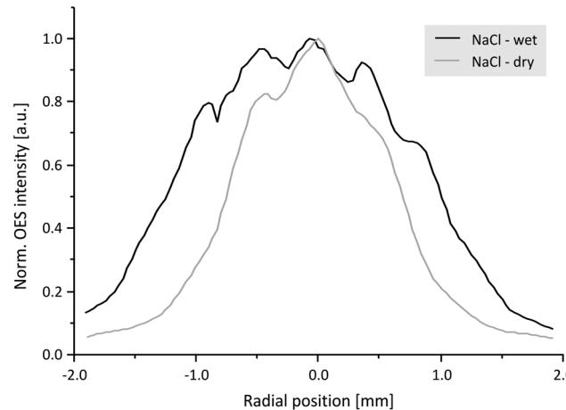
Fig. 5 Radial emission profiles for sodium chloride under dry and wet plasma conditions at the axial position of maximum emission. The profiles were integrated axially over a width of 0.3 mm and normalized with respect to maximum intensity values.
