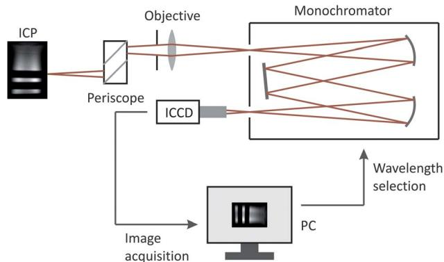
Fig. 2 Sketch of the monochromator-based 2D imaging setup used for OES mapping of an ICP.
