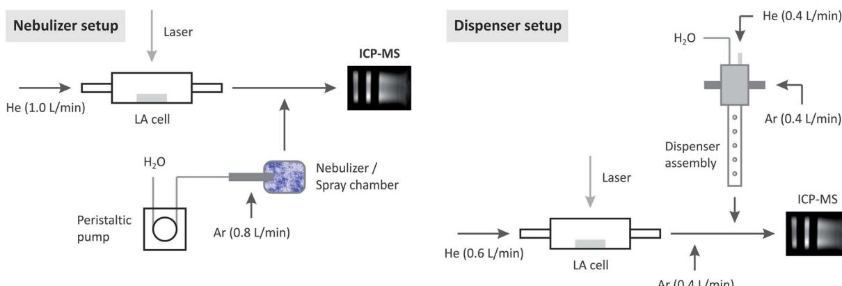
Fig. 3 Left panel: LA and carrier gas wetting using a nebulizer and spray chamber. Right panel: LA and carrier gas wetting using a micro-droplet dispenser.
