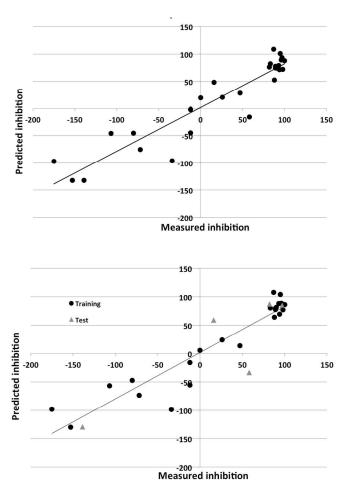
**Figure 5**. The observed versus predicted corrosion inhibition for 2024 alloy for the nonlinear model using DRAGON descriptors. Top panel: model for entire data set. Bottom panel: data set split into training (circles) and test (triangles) sets.
