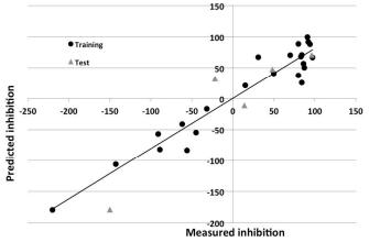
**Figure 3**. Observed versus predicted corrosion inhibition for 7075 alloy for the nonlinear model using DRAGON descriptors. Top panel: model for entire data set. Bottom panel: data set split into training (circles) and test (triangles) sets.
