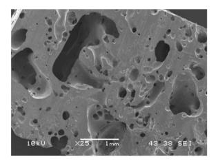
Figure 1: Scanning electron micrograph of acrylated epoxidised soybean oil based macroporous polymers manufactured by mechanical frothing. Obtained from Lee et al.<sup>36</sup> with kind permission from the Royal Society.
