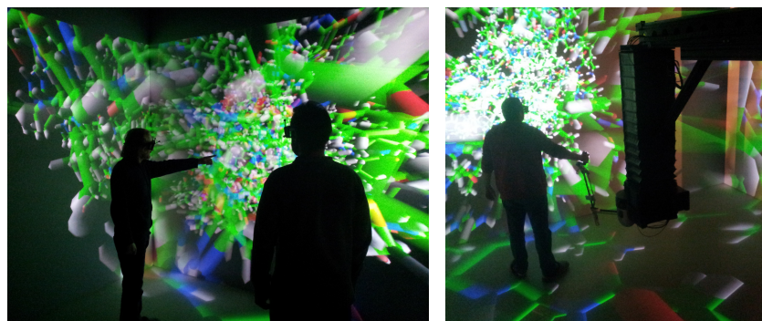
Fig. 7 (a) Two users in our collaborative Cave-like system, each with their own head-tracked 3D point of view, allowing pointing to discuss about a shared 3D object. (b) Our advanced haptic device allows users to access the whole workspace of the immersive system.
