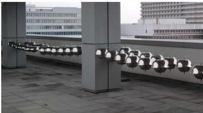
Polyurethane foam passive air sampler shows large inter-compound variability in sampling performance for semivolatile organic compounds in outdoor environment.
