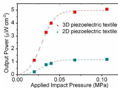
Using “3D-spacer” technology, we demonstrate novel all-fibre piezoelectric fabric power generators. The single-structure generator comprises 80%  $\beta$ -phase PVDF spacer monofilaments interconnected between woven Ag/PA66 electrodes. The structure provides power density of 1.10-5.10 $\mu\text{Wcm}^{-2}$  at applied impacts of 0.02-0.10MPa, nearly five times higher than existing 2D structures.
