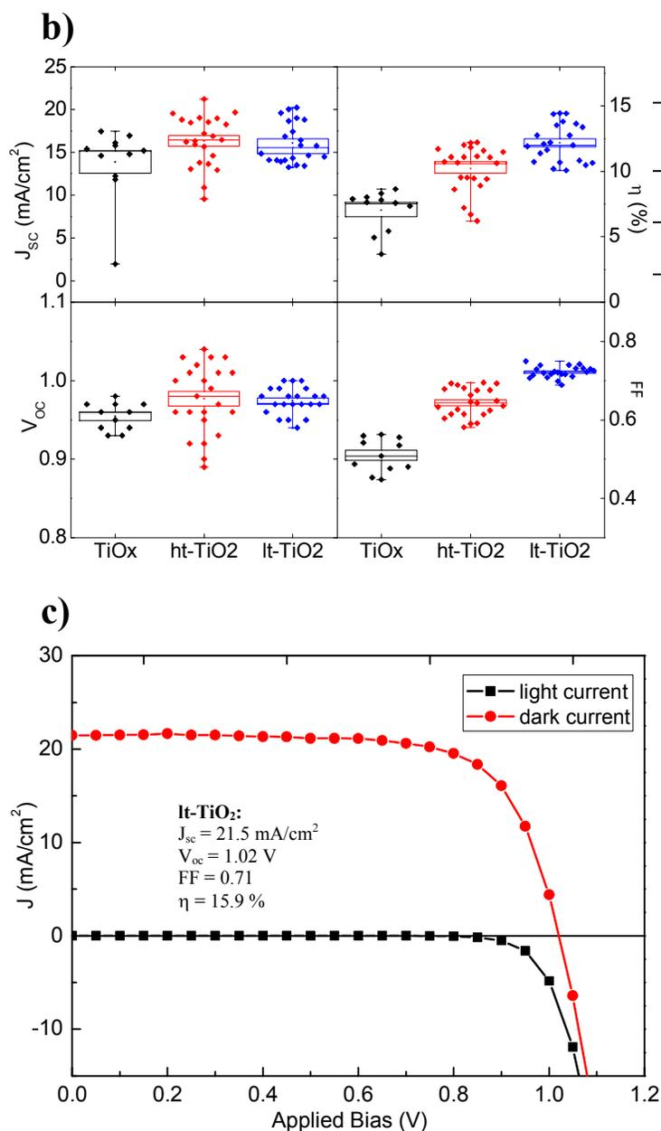
**Figure 2.** (a) Current-voltage characteristics of the best performing solar cells made with amorphous (TiO<sub>x</sub>), high-temperature (ht-TiO<sub>2</sub>) and low-temperature (lt-TiO<sub>2</sub>) processed compact layer; (b) photovoltaic parameters extracted from current-voltage measurements of a series of solar cells with the different compact layers; (c) record lt-TiO<sub>2</sub> solar cell performance obtained by increasing perovskite film thickness.
