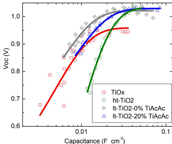
Figure 3. Open circuit voltage against the differential capacitance.
