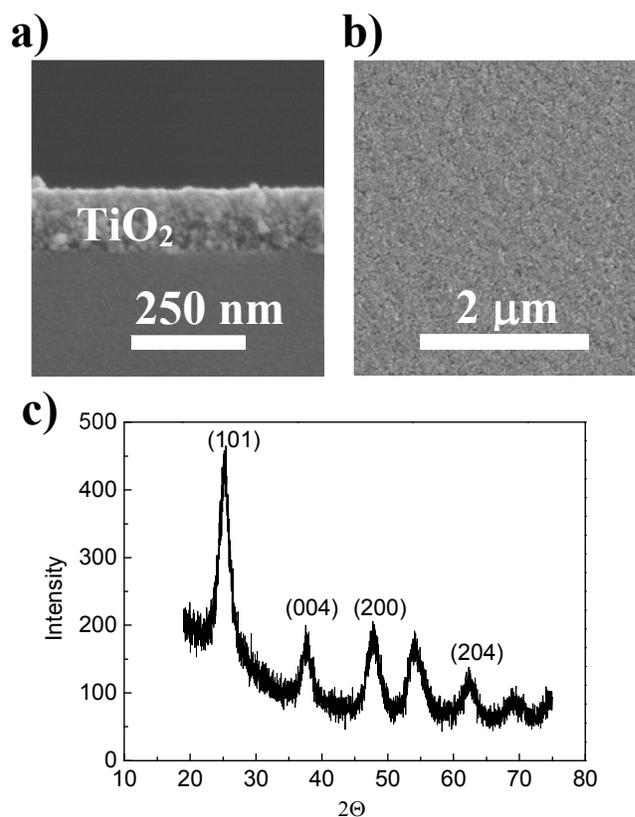
**Figure 1.** (a) Cross-sectional image of 3.54 weight% TiO<sub>2</sub> NPs spin-coated on glass, thickness: 100-120 nm; (b) top surface image of lt-TiO<sub>2</sub>; (c) X-ray diffraction spectrum of TiO<sub>2</sub> nanoparticles powder sample.
