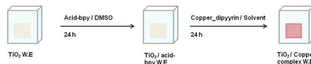
Fig. 7 In situ protocol for producing a copper complex on the surface of TiO_2 working electrode.
