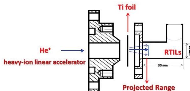
Fig. 2 The equipment for the irradiation of ionic liquid using  $\text{He}^+$  beam.
