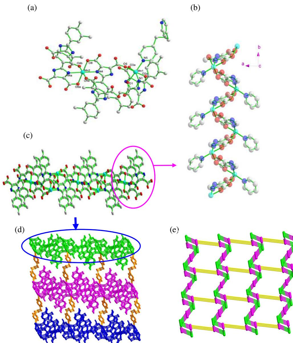
Figure 1. (a) View of the coordination environments of the Mn centers in **1**. (b) One-dimensional meso-helical chain. (c) Side view of the two-dimensional sheet. (d) Three-dimensional structure of **1**. (e) Schematic representation of **1**.
