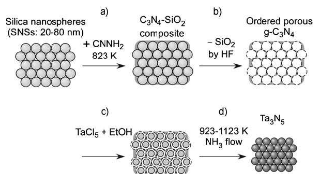
Scheme 3. Illustration of the synthesis of ordered porous \text{g-C}_3\text{N}_4 and regularly arranged \text{Ta}_3\text{N}_5 nanoparticles by using close-packed silica nanospheres as the primary
