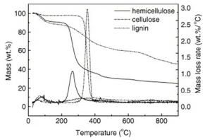
Figure 2 Pyrolysis curves of hemicellulose, cellulose, and lignin from TGA. (Adapted with permission from Yang et al., *Fuel*, 2007, **86**, 1781-1788.<sup>77</sup> Copyright 2007 Elsevier)
