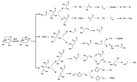
Figure 4 Reaction pathways for secondary decomposition of anhydrosugars (especially levoglucosan). (Adapted with permission from Shen et al., *Bioresour. Technol.*, 2009, **100**, 6496-6504.<sup>75</sup> Copyright 2009 Elsevier)
