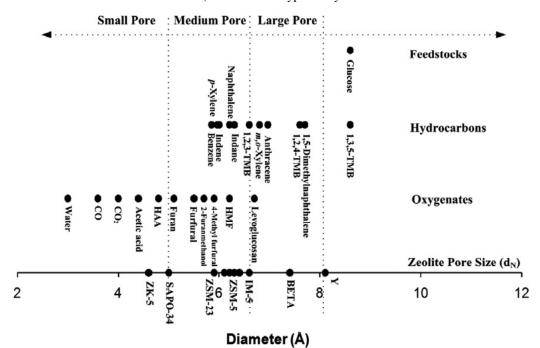
Figure 8 Schematic comparison of zeolite pore diameter and kinetic diameter of feedstocks, oxygenates, and hydrocarbons in CFP of biomass.(Adapted with permission from Jae et al., *J. Catal.*, 2011, **279**, 257-268.<sup>246</sup>. Copyright 2011 Elsevier)
