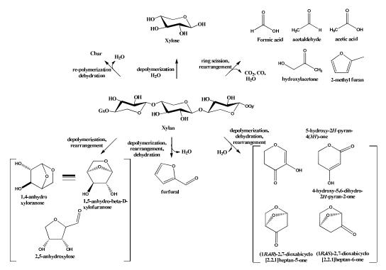
Figure 5 Proposed reaction scheme of hemicellulose pyrolysis. (Adapted with permission from Patwardhan et al., *ChemSusChem*, 2011, **4**, 636-643.<sup>78</sup> Copyright 2011 John Wiley and Sons)
