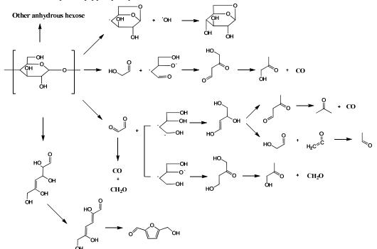
Figure 3 Reaction pathways for the direct decomposition of cellulose molecules. (Adapted with permission from Shen et al., *Bioresour. Technol.*, 2009, **100**, 6496-6504.<sup>75</sup> Copyright 2009 Elsevier)
