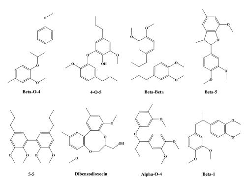
Figure 6 Common phenylpropane linkages in lignin. (Adapted with permission from Chakar et al., *Ind. Crop and Prod.*, 2004, **20**(2), 131-141.<sup>121</sup> Copyright 2004Elsevier)
