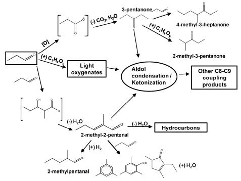
Figure 7 Proposed reaction pathway of propanal over ceria-zirconia catalyst.(Adapted with permission from Gangadharan et al., *Appl. Catal., A*, 2010, **385**, 80-91<sup>168</sup>. Copyright 2010 Elsevier)
