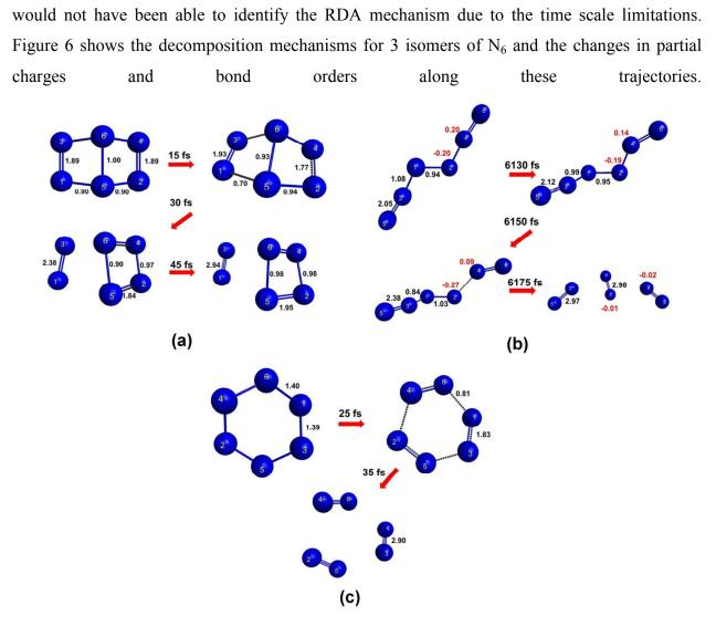
Fig.6: NBO bond orders and partial charges along the decomposition dynamics of 3 isomers of  $N_6$ . Bond orders are in black and partial charges are in red. Panel (a) shows the Dewar benzene isomer. Following the bond orders on-the-fly revealed a two step decomposition mechanism. The first step is shown and found to be a retro Diels Alder mechanism. Panels (b) and (c) show the concerted decomposition mechanisms found for 2 additional isomers.
