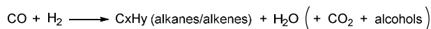
Figure 1. General scheme for FT synthesis reaction from syngas to a range of potential products.
