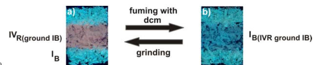
Fig. 9 Reversible stimuli-responsive luminescence of \text{I}_B : a) red emitting \text{IV}_R(\text{ground } \text{I}_B) obtained by grinding the blue luminescent \text{I}_B and b) reversion to blue luminescent \text{I}_B(\text{IV}_R \text{ ground } \text{I}_B) after fuming \text{IV}_R(\text{ground } \text{I}_B) with dichloromethane
