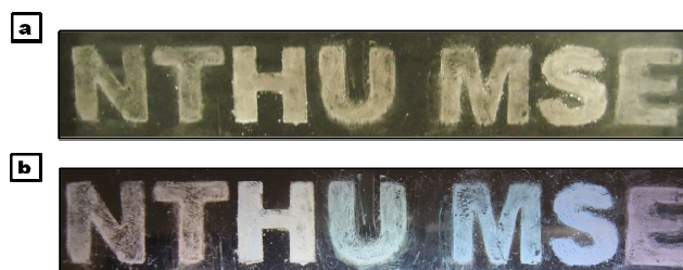
Fig. 5 Photographs of transparent plastic slides which were coated with various-sized spheres by doctor-blade. (a) All spheres synthesized with different concentration of HMTA (40-140 mM) have white color which is similar to general ZnO powders. (b) When turn on a back light, multicolored words could be observed through the transparent plastic slides by Mie scattering at scattering angle \theta > 0^\circ (from left to right, red (S4), orange (S6), yellow (S8), green (S10), cyan (S12), blue (S13), and purple (S14), respectively).
