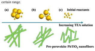
75 Fig.7 Schematic illustration of different dosage of TEA solution into Ti precursor, which will grow into pre-perovskite PbTiO<sub>3</sub> nanofibers of different sizes via hydrothermal reaction (the yellow particles: initial reactants; the green fibers: pre-perovskite PbTiO<sub>3</sub> nanofibers).
