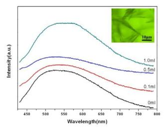
Fig.8 PL spectra of sample 1-4 excited by 410 nm wavelength Xenon lamp at room temperature. The upper inset shows that the nanofibers in <sup>10</sup> sample-1 present obvious green light.
