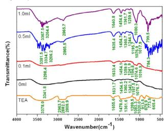
Fig.5 FTIR spectra of the amorphous powder precursors prepared by the 30 sol-gel and subsequent freeze-drying process (the bottom curve represents the FTIR spectrum of pure TEA, the upper ones show the FTIR spectra of modified amorphous precursor in sample 1-4).
