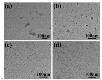
Fig.6 TEM images of the amorphous powder precursors prepared by the modified sol-gel process and the freeze-drying treatment. (a)- (d): sample 1-4, respectively.
