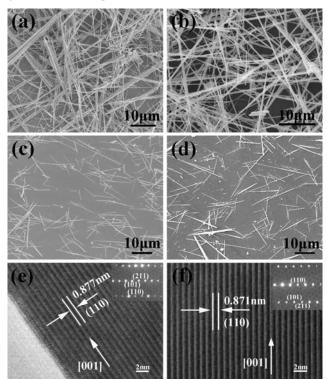
Fig.3 SEM images of pre-perovskite PbTiO3 nanofibers. (a)- (d): sample 1-4, respectively. High-resolution TEM (HRTEM) images of preperovskite PbTiO<sub>3</sub> nanofibers, (e): sample-1, (f): sample-4. The insets in 10 (e) and (f) show the selected area electron diffraction pattern.
