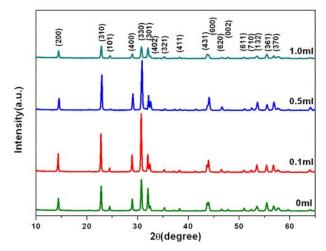
Fig.2 XRD patterns of pre-perovskite PbTiO<sub>3</sub> nanofibers (sample 1-4) by adding different amount of TEA solution.
