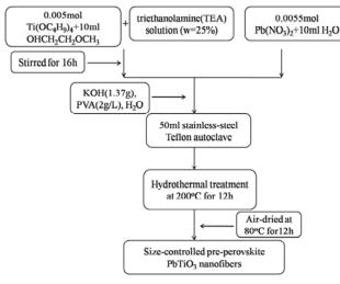
Fig.1 The flowchart for the synthesis of pre-perovskite PbTiO<sub>3</sub> nanofibers by the modified sol-gel process and the PVA-assisted hydrothermal <sup>30</sup> reaction
