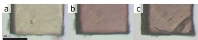
Figure 4. Images of a UBMOF-1 single crystal: (a) before exposure to UV light, (b) after irradiation with 365 nm light, and (c) after irradiation with visible light for >2 hours
